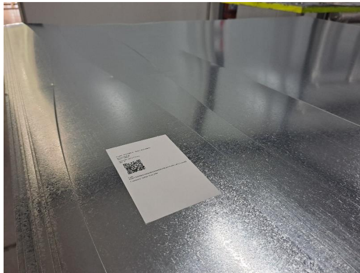
Example: Sticker stuck on the pre-cut elbow plate.
